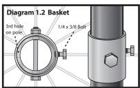
3/8" hex bolt into the threaded hole on the basket and tighten against the pole.
