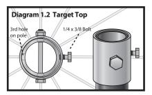
as you put the target top onto the pole. Align target top with the threaded hole on the **opposite** side of the pole from the third hole in the pole. Insert 5/16" x 2 3/4" hex bolt through target top and pole and tighten nut with wrench. Insert the 1/4" x 3/8" hex bolt into the threaded hole on the target top and tighten against the pole.
